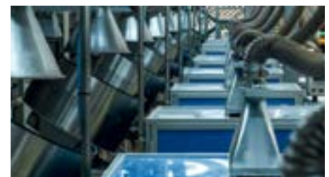
SVE ( Sealing Verification System) An individual screening technology that ensures the sealing capacity of each natural cork stopper.
